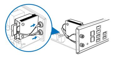
3. Replace the bolt on the connector to secure the antenna connector and the I/O shield in place.
